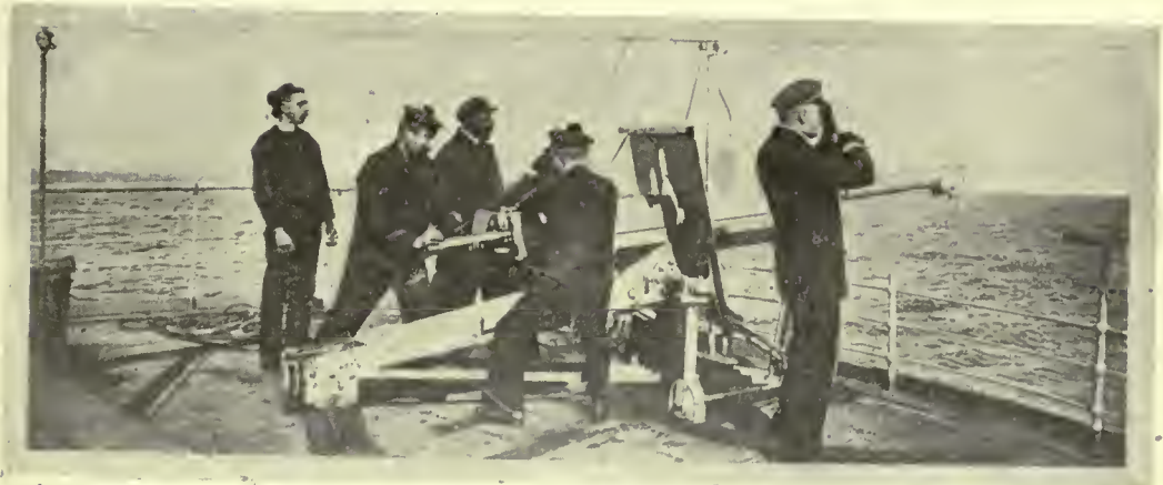
FRENCH ANTI-SUBMARINE 75mm. GUN IN A MERCHANT SHIP.
