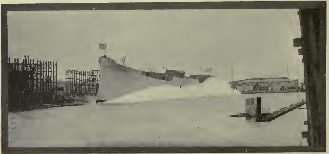
THE LAUNCHING SIDEWAYS OF THE STEAMER NANTHALA At Messrs. Schaw-Batcher's yard at South San Francisco on Independence Day, 1918.
